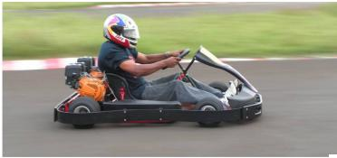
The KnK Genesis Pro is fitted with a floor mounted 8-litre petrol tank and the red body parts set it apart from the other Genesis models. Engine cowls are an optional fitting.
